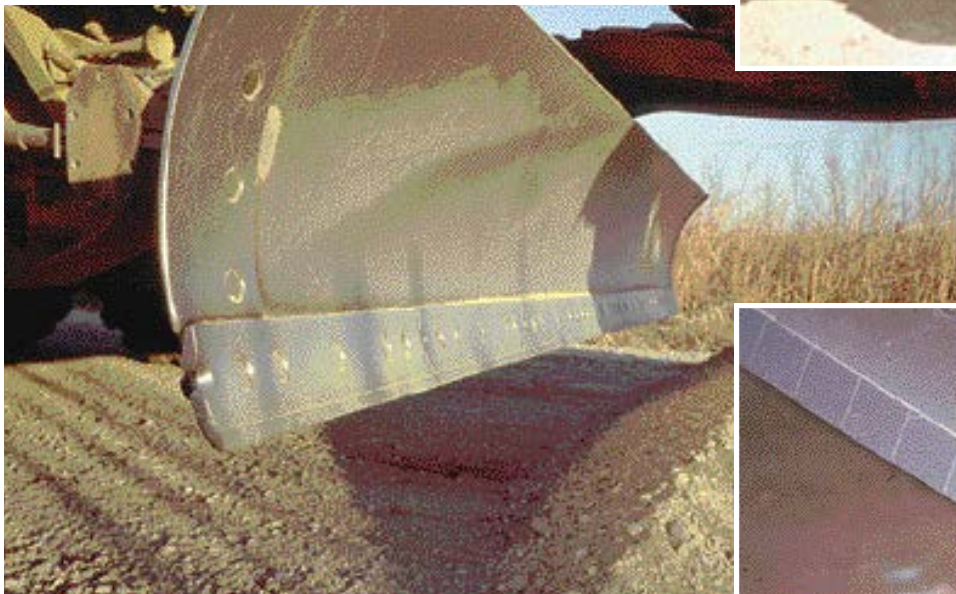
An example of a carbide-faced blade after 650 hours of use. The center sections had been exchanged with the outer sections once during this time.
